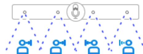
Next-generation beamforming microphone array
