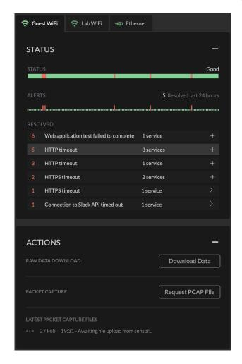
HPE Aruba Networking UXI Sensor use dynamic packet captures that are uploaded to the cloud when issues are detected. The packet capture data is invaluable for troubleshooting issues in depth and arriving at root cause without having to visit the site. Reported data includes: connectivity, throughput, latency, jitter, packet loss, web server response time, web application transaction time and VoIP MoS.
